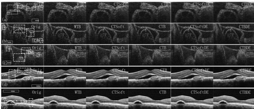
**Fig. 6.** (a)-(e) are the denoised OCT images based on five algorithms. The first column is the original noisy images, the algorithm used is showed on the top right corner. The images (d) and (c) come from the <http://www.optos.com/en/Professionals/Image-library/>
